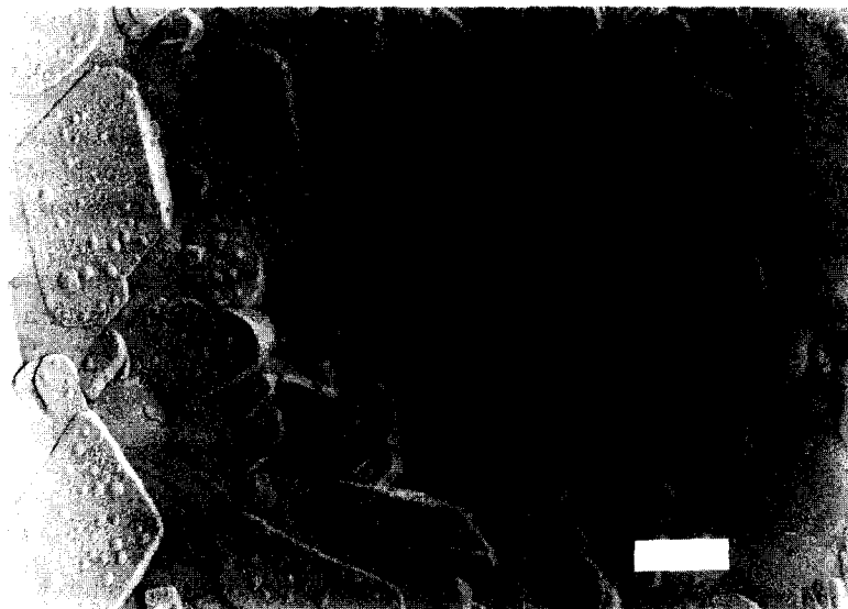
Fig. 6. Transmission electron micrograph of a 10% tripalmitate gel stabilized by 1.2% S100 only (10 times homogenized at 800 bar). The fractures were decorated with water. The bar indicates 230 nm.
